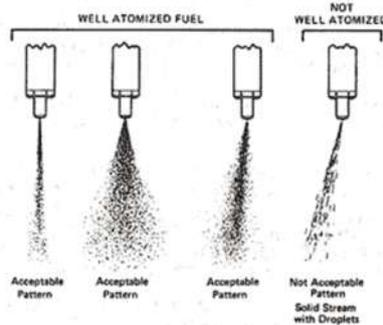
Quite often these older oil burners delivered a shot of fuel with a poor and ill-defined spray pattern that was either too rich (most often) or too lean. This resulted in either a rich belch of sooty black smoke or insufficient power or a struggling vehicle. To make matters worse, the low pressure fuel had to be injected into a pre-chamber to insure proper atomisation of the before it could mosey into the main combustion chamber to do its work.
