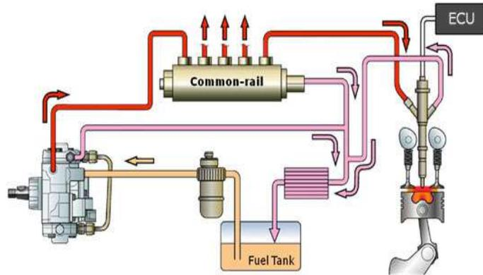
In addition to timing control, the short duration, high pressure injections allow a finer and more accurate spray pattern that also supports better and more complete atomization and combustion.
